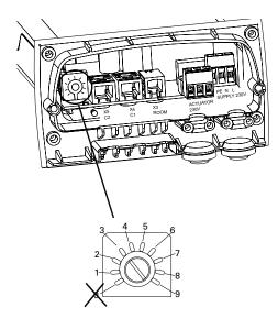
Each unit should have a unique ID on its SIReB1/B2/B1EC card.
