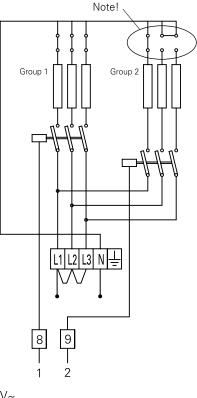
230V~ Step 1: 4,5kW Step 2: 6,8kW
