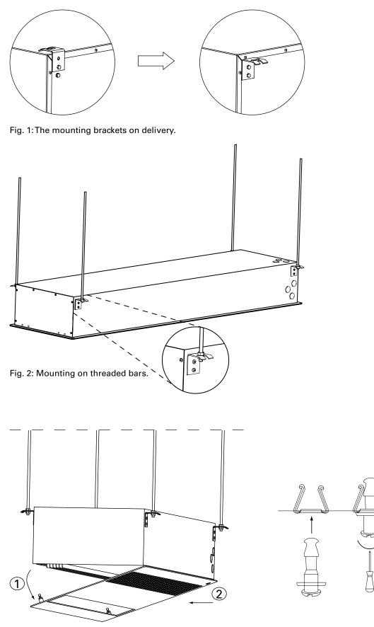
Fig. 3: Removal of bottom plate
