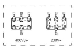
To choose output - connect the contactors as outlined in the wiring diagrams below.
