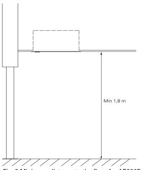
Fig. 5 Minimum distance to the floor for AR200E.
